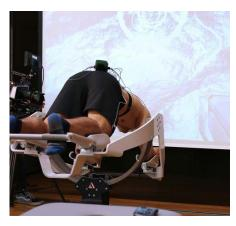
Icaros is a training device that turns the core 'plank' muscle exercise into a more dynamic one by making it mobile. The user lies horizontally in a prone position with forearm support on a motion platform specially equipped with movement sensors that are able to detect any changes in the user's direction and translate them into virtual reality (VR). VR glasses and a large screen give the user a real
