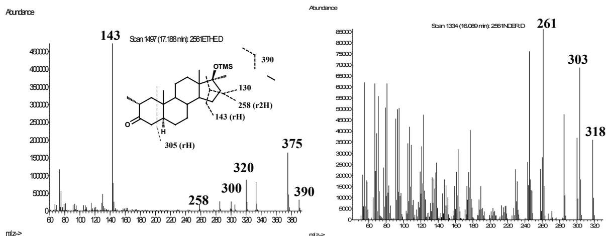
Figure 6: Mass spectrum of synthesised  $2\alpha,17\alpha$ -dimethyl- $5\alpha$ -androstan- $3\alpha$ -one- $17\alpha$ -ol, TMS-ether (left) and underivatised (right) and proposed fragmentation pathways.
