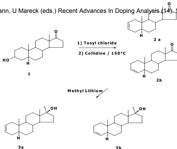
Figure 2: Scheme of chemical synthesis of 17 $\alpha$ -methyl-5 $\alpha$ -androst-2-en-17-ol (DMT) (3a) from epandrosterone (1) via 5 $\alpha$ -androst-2-en-17-one (2a; major)
