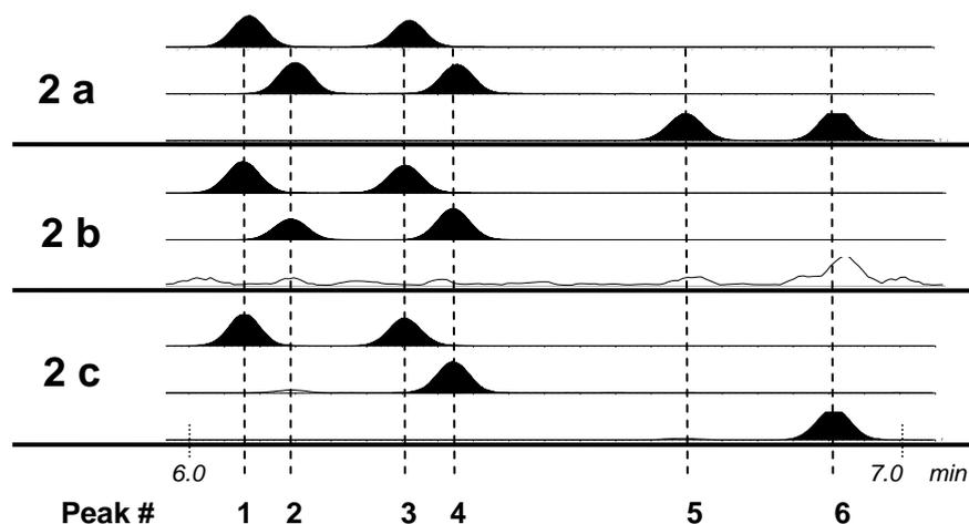
Figure 2. Ion chromatograms of a calibrator (2 a), an amphetamine positive sample (2 b) and a selegilin positive sample (2 c). Peak 1-6 corresponds to (D-) amphetamine-D8 TFAP, (D-) amphetamine TFAP, (L-) amphetamine-D8 TFAP, (L-) amphetamine TFAP, (D-) methylamphetamine TFAP and (L-) methylamphetamine TFAP, respectively.
