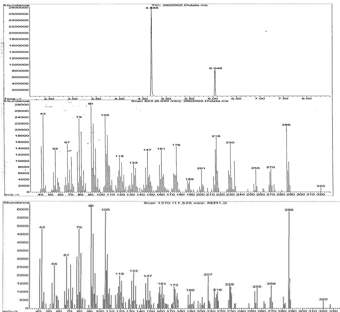
**FIG 12:** Chromatogram and Mass spectrum of compound from Hemapopin (upper traces) and the mass spectrum from Epistane (lower trace).
