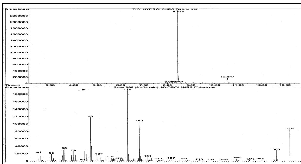
**FIG. 6** Mass spectrum of underivatised alcohol (A) at 8.44 min.
