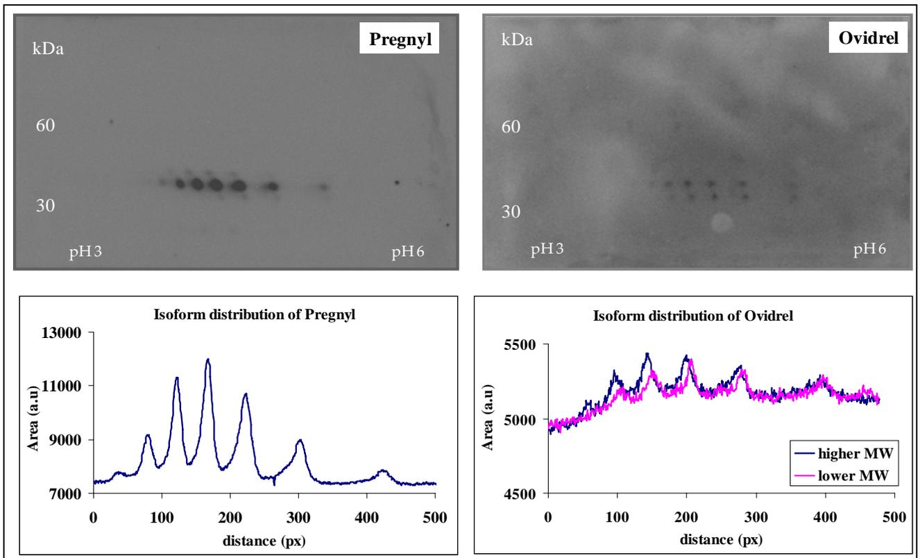
**FIG 3.** 2D-gels obtained using a pH gradient from 3 to 6 in the electrofocusing step.
