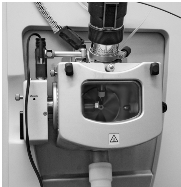
Fig.1. Dual ESI/APPI source configuration for the Exactive mass spectrometer
