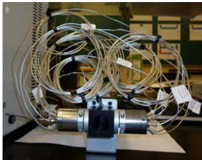
Figure 2. Fraction collector made with two eight-port valves provided with a multiposition microelectric valve
