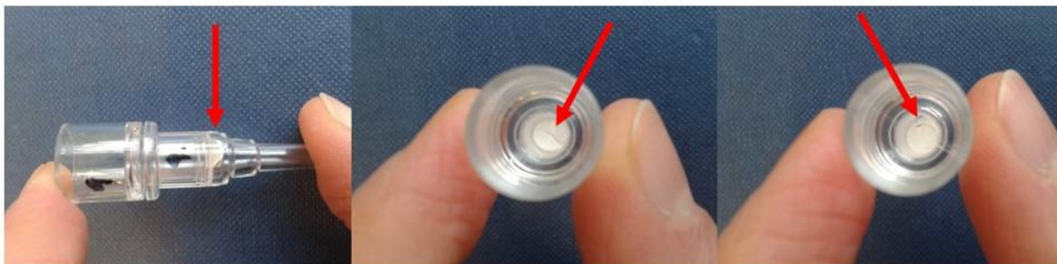
Figure 4: Defective monoliths in the MAIIA columns (monolith not properly placed inside the column, broken monolith, or monolith with little holes).
