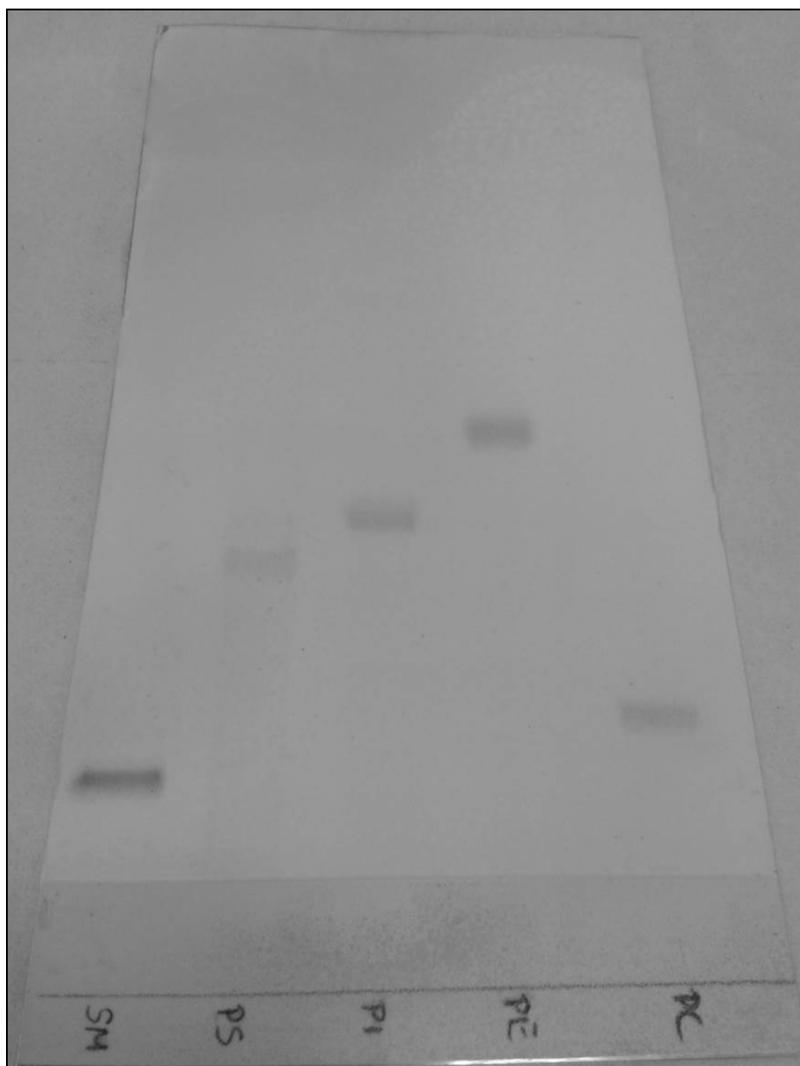
Figure 1: TLC plate with separated lipid standards (SM = Sphingomyelin, PS = Phosphatidylserine, PI = Phosphatidylinositol, PE = Phosphatidylethanolamine, PC = Phosphatidylcholine)
