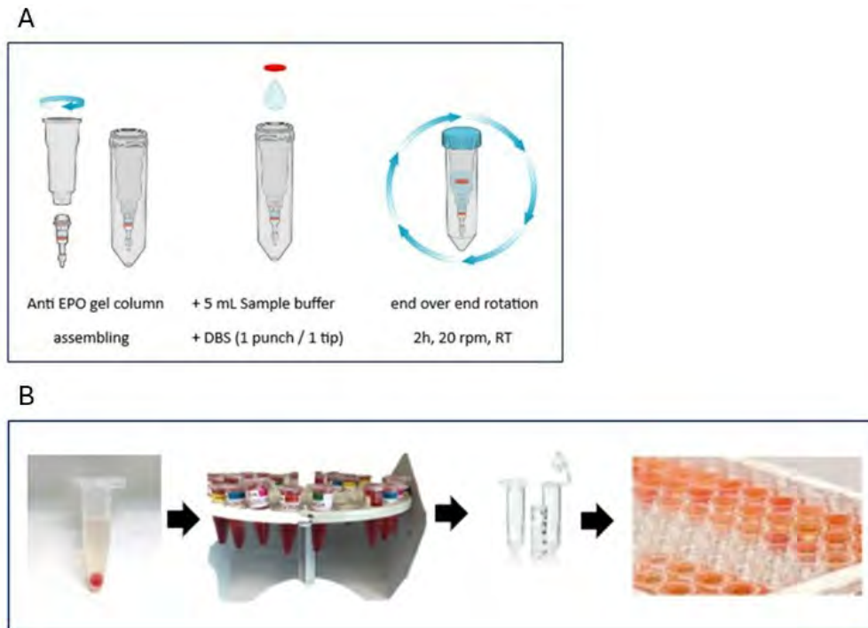
Figure 2. A: MAIIA EPO Purification gel kit for blood ( https://maiiadiagnostics.com/wp-content/uploads/2024/04/DfU-EPGK-B-2024.pdf ). B: PBS extraction and immunopurification with ELISA
